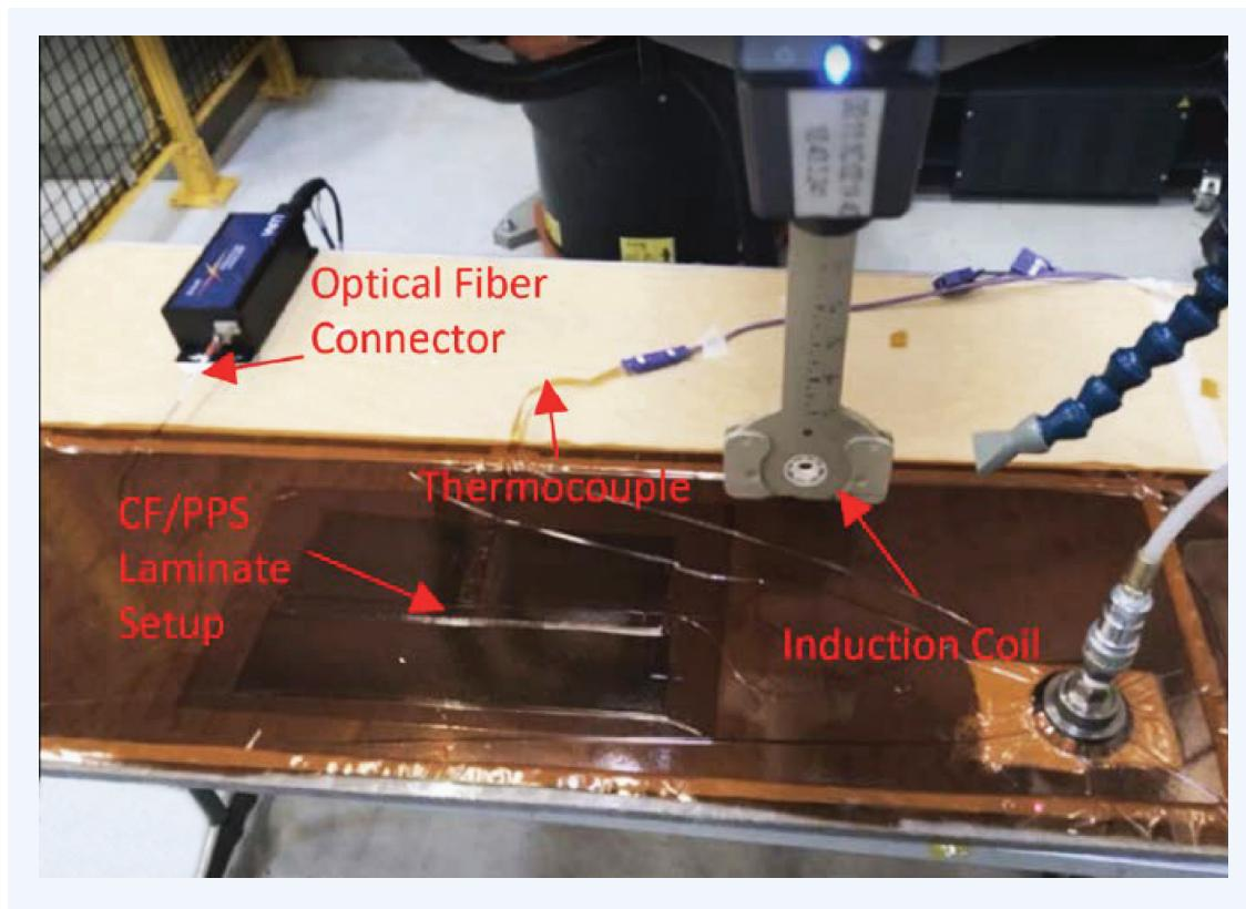
Figure 3. Induction Welding Setup
