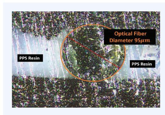
Figure 6. Microscopy of PPS Coating melted off in Bond Line
