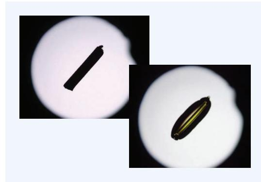
Figure 7. PPS coated fiber optic before (left) and after (right) melting
