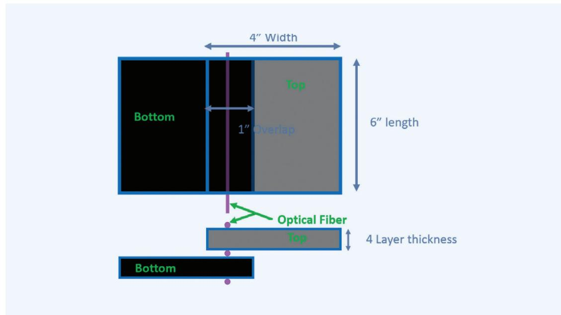
Figure 4. Laminate Welding Configuration
