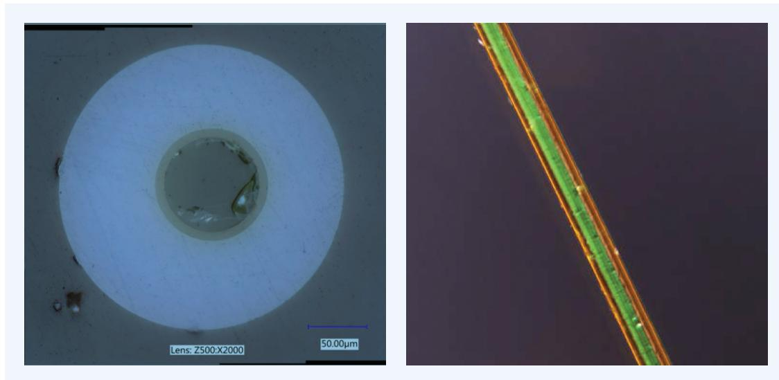
Figure 2. (Left) PPS Coated HD-FOS Sensor
