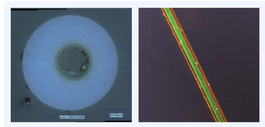
Figure 2. (Left) PPS Coated HD-FOS Sensor (Right) HD-FOS sensor with Polyimide Coating
