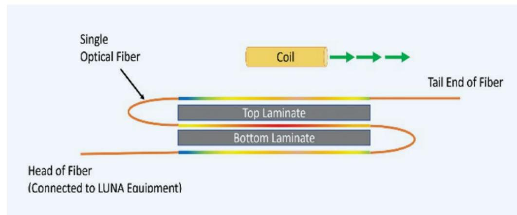
Figure 5. Optical Fiber placement and sensor selection along length of fiber for data collection
