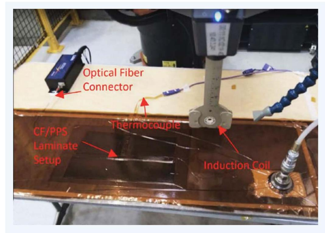
Figure 3. Induction Welding Setup
