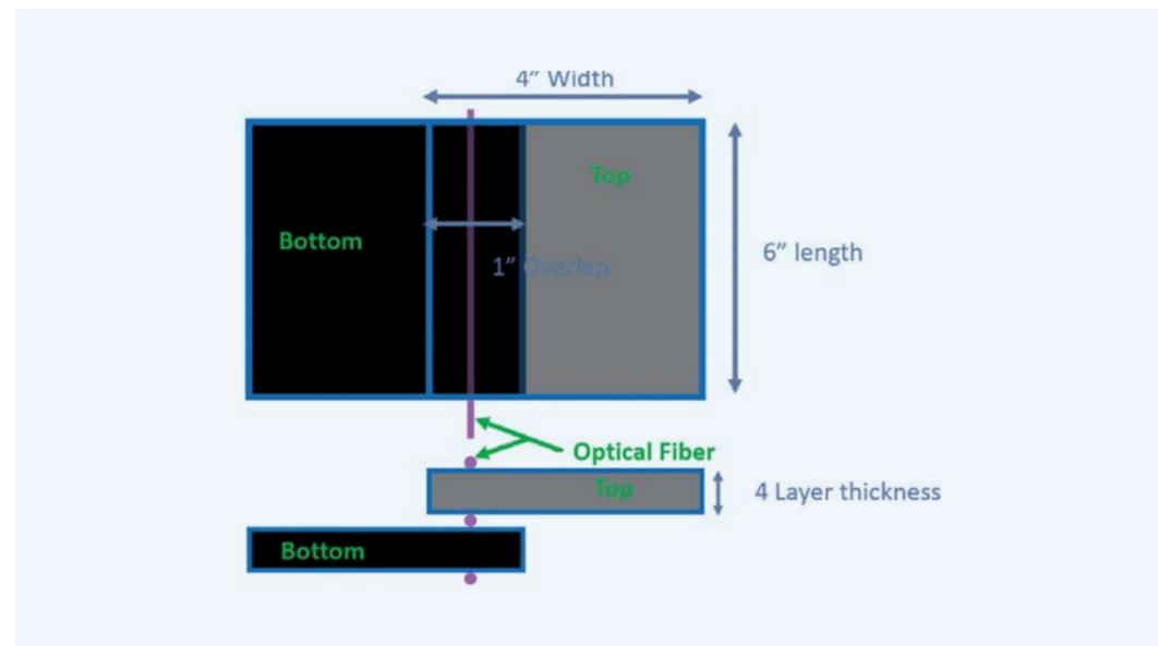
Figure 4. Laminate Welding Configuration
