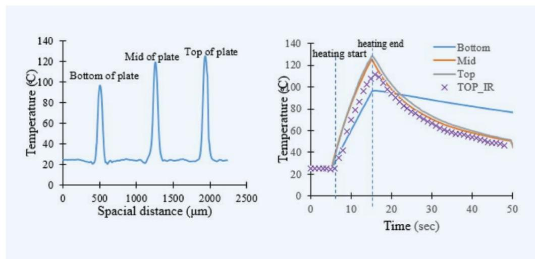
Figure 8. In-process monitoring of temperature (left) temperature values along fiber length (right) temperature values over time
