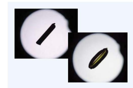
Figure 7. PPS coated fiber optic before (left) and after (right) melting
