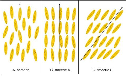
**Figure 2:** Diagram showing the arrangement of mesogen molecules within liquid crystal types. Liquid crystal forms exhibit directional alignment of their molecules and are anisotropic. **(A)** Nematic liquid crystal showing orientational order, **(B)** smectic A liquid crystal form, and **(C)** smectic C liquid crystal form. B and C possess orientational and positional order.
