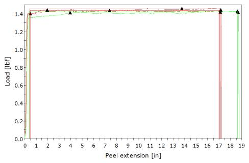
Figure 3. Load versus Extension for PHS2 sample in tear tests at 23°C (three replicates).
