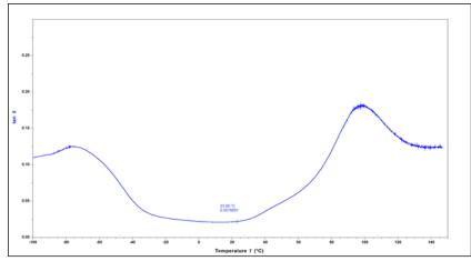
Figure 4. Tan  $\delta$  for recovered HS as a function of temperature.
