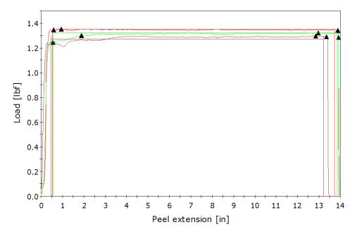
Figure 2. Load versus Extension for PHS1 sample in tear tests at 23°C (three replicates).
