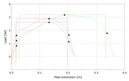
Figure 1. Load versus Extension for HS sample in tear tests at 23°C (three replicates).
