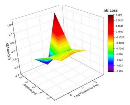
Figure 5:  $\Delta E_{Loss}$  (20°C - 30°C) vs Amplitude and Frequency for HS3
