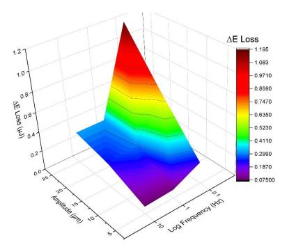
Figure 3:  $\Delta E_{Loss}$  (175°C - 185°C) vs Amplitude and Frequency for HS2
