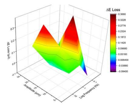
Figure 6: △E<sub>Loss</sub> (210°C - 220°C) vs Amplitude and Frequency for HS3
