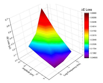
Figure 4: △E<sub>Loss</sub> (175°C - 185°C) vs Amplitude and Frequency for HS3
