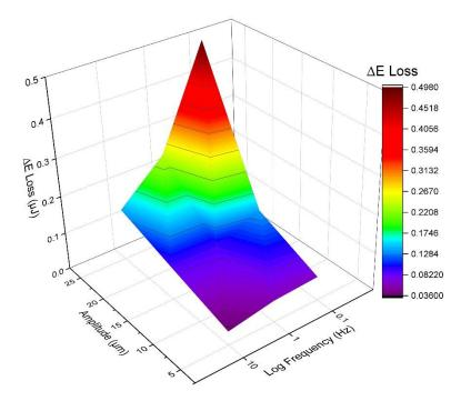
Figure 2: △E<sub>Loss</sub> (175°C - 185°C) vs Amplitude and Frequency for HS1
