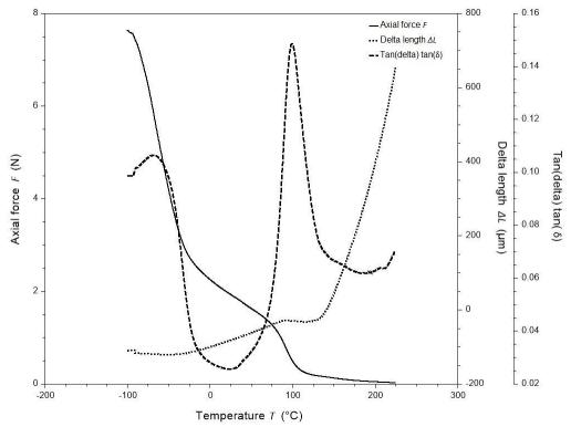
Figure 1: Temperature Ramp @ 1Hz Frequency and 15 µm Amplitude for HS1
