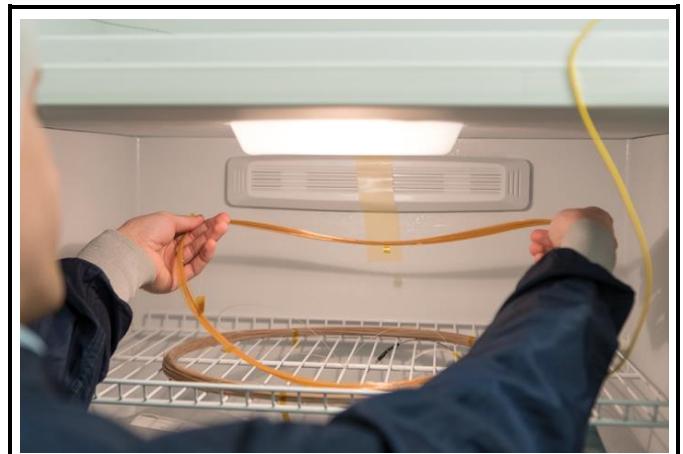
Figure 5: Testing scheme for sub-zero temperature measurements showing placement of fiber optic coils in the sub-zero freezer.
