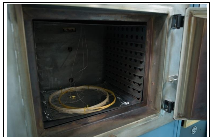
Figure 6: Testing scheme for elevated temperature cycling measurements showing placement of fiber optic coils in the furnace.
