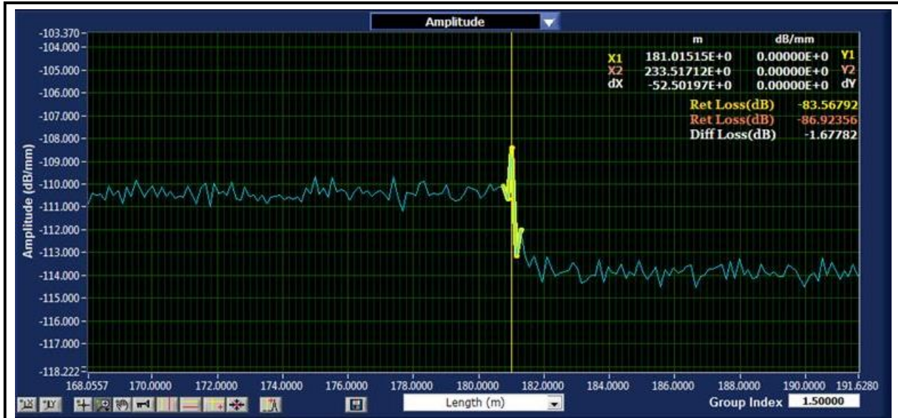
Figure 9: Representative image showing the determination of the positioning of the spring clamp on the fiber by artificially inducing attenuation by bending (PEEK coated fiber shown).
