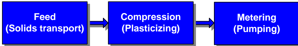
The major functions of the extruder screw
